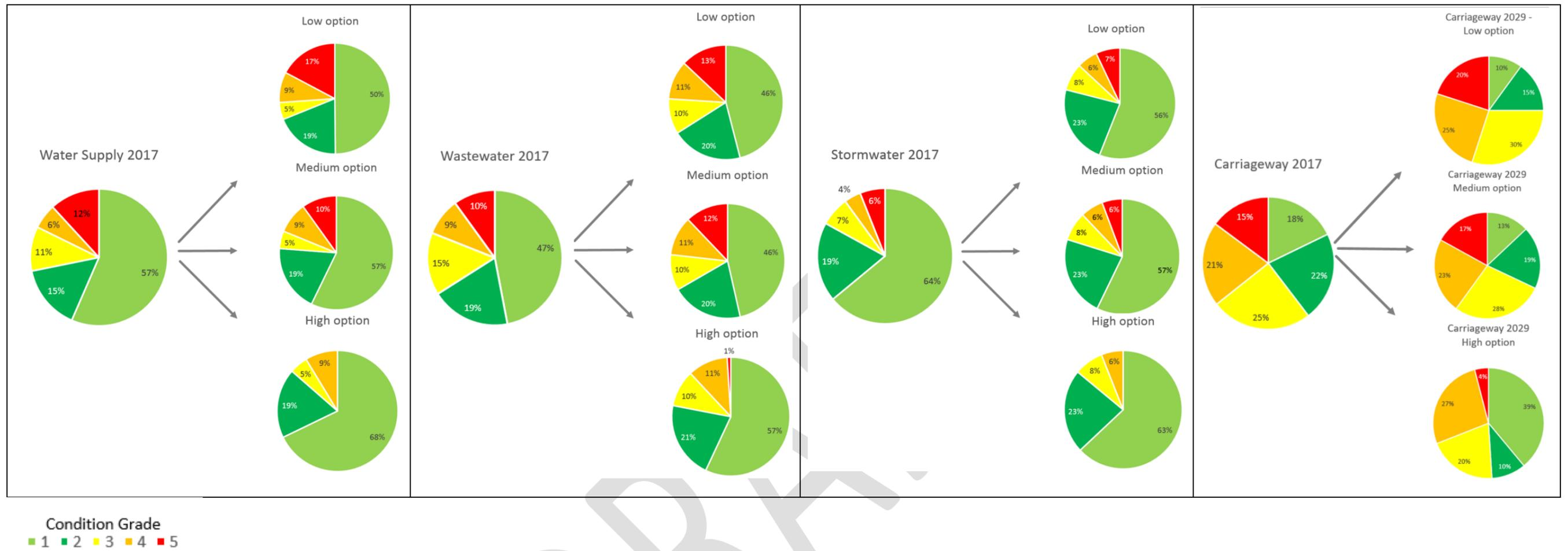
For water supply, wastewater and stormwater pipes: 1 – as new, 5 – expected to fail in 1-2 years. For carriageway: 1 – excellent, 2 – good, 3 – average, 4 – poor, 5 – very poor.
